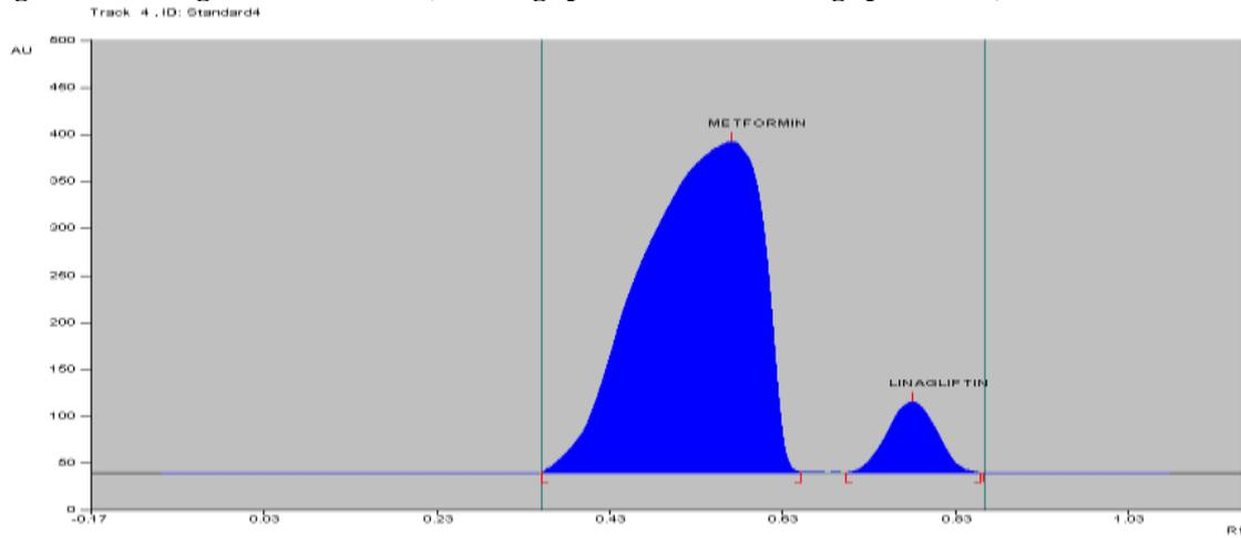
**Fig 8. Chromatogram of standard (16000 ng/spot of MET and 80 ng/spot LINA)**
