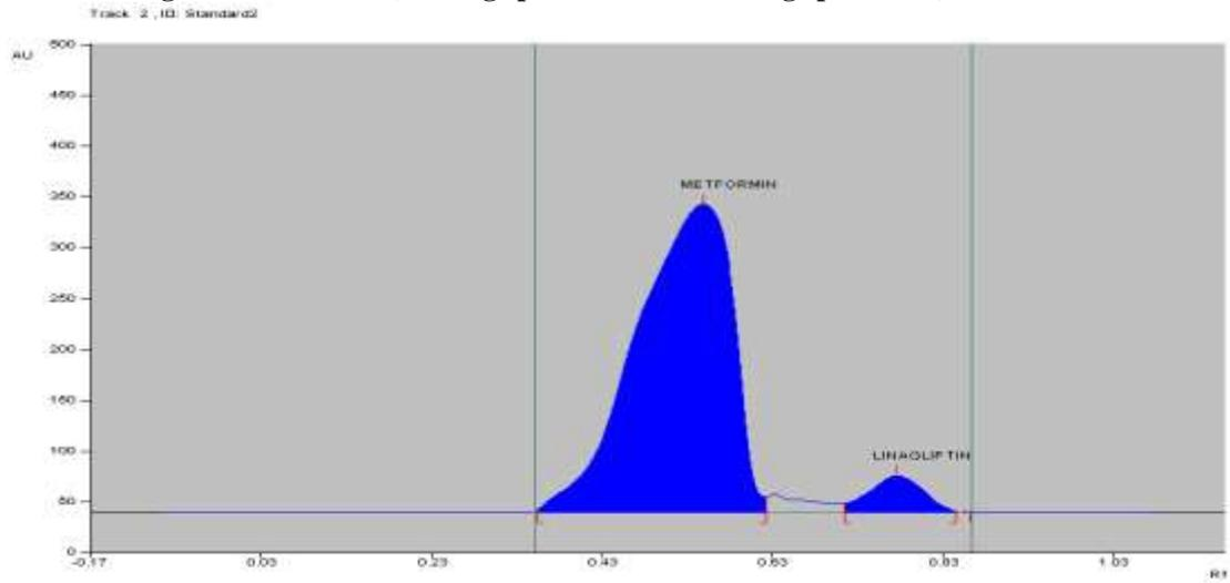
**Fig 6. Chromatogram of standard (8000 ng/spot of MET and 40 ng/spot LINA)**
