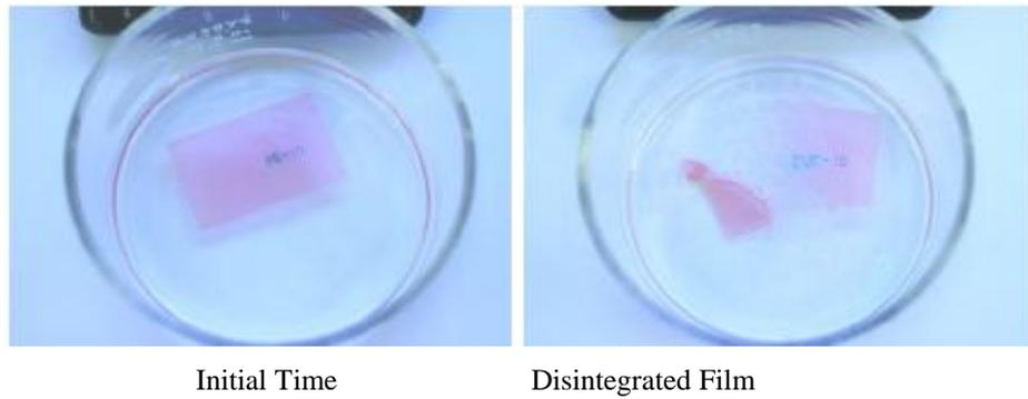
Figure 1: Disintegration of the film
