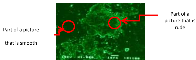
Figure 2. Cross-section of bioplastic by comparison of chitosan and cellulose pulp 5:10 on a scaled up 1000x
